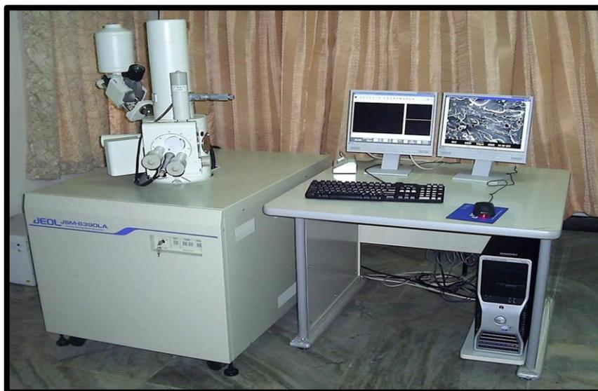
*Figure 2.9: Field emission gun- scanning electron microscope.*
