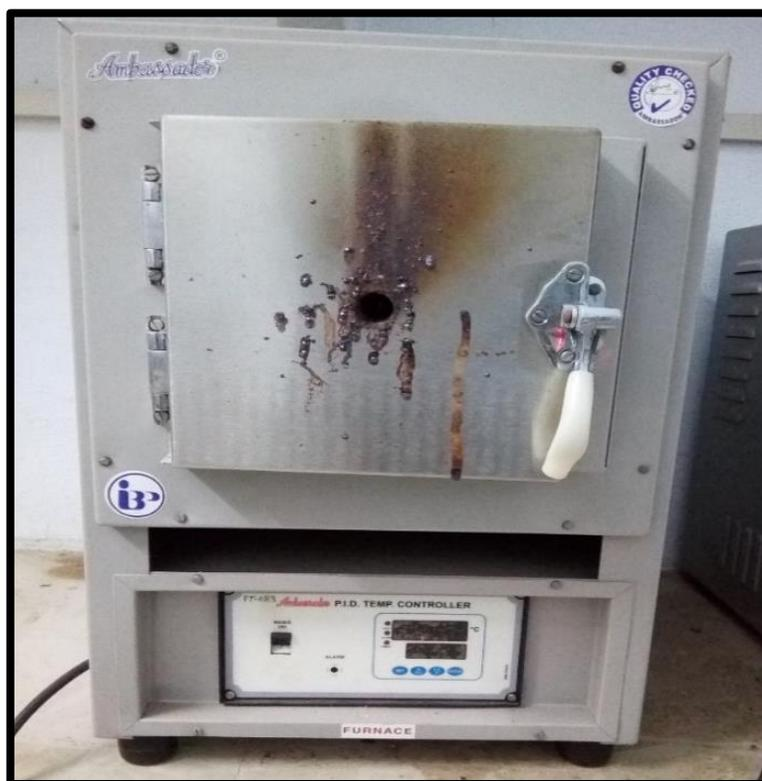
*Figure 2.1: Muffle Furnace*
