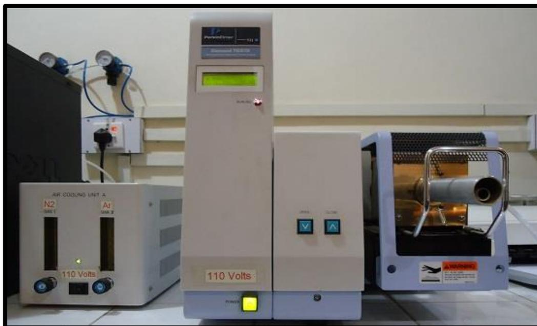
**Figure 2.5: Thermogravimetric/differential thermal analyzer**
